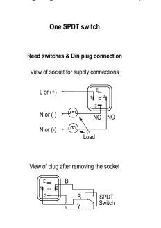
R=Red, B=Black, Y=Yellow, L=Live or +ve supply, N=Nutral or -ve supply \* Body to be suitably earthed while using gauge + switch.
