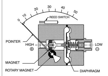
If pressure exceeds the rated maximum pressure, "O" rings & diaphragm inside the pressure chamber, will be damaged. If maximum operating pressure is within the allowable limit of 35 bar, but the differential pressure exceeds instrument range, there will be no damage to the instrument. Pointer will only go the extreme right end of the scale.
