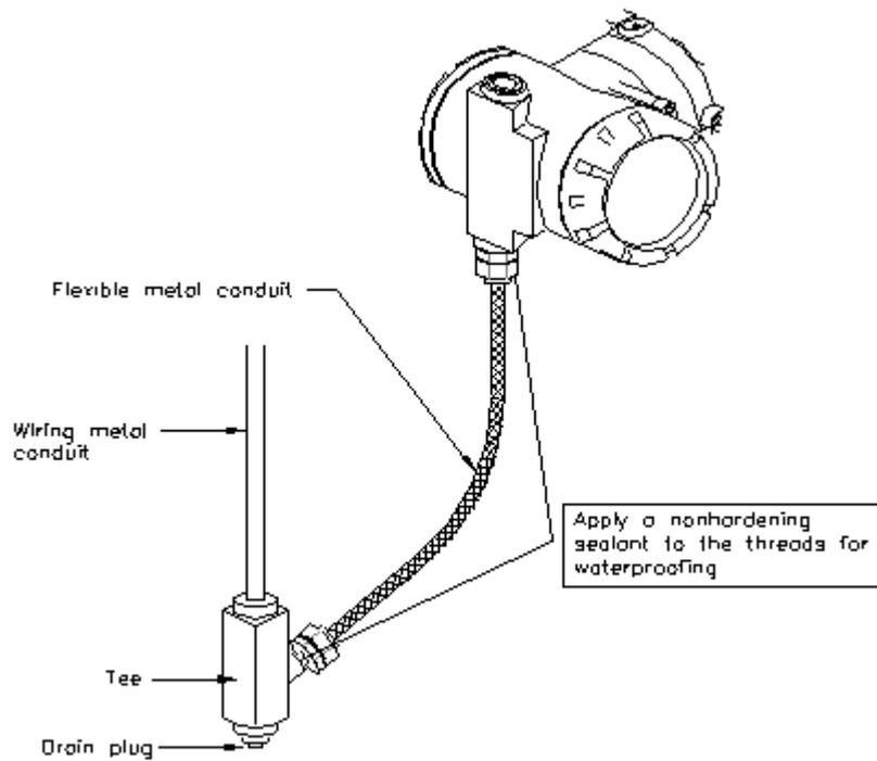
[Figure 4 Typical Wiring Using Flexible Metal Conduit]
