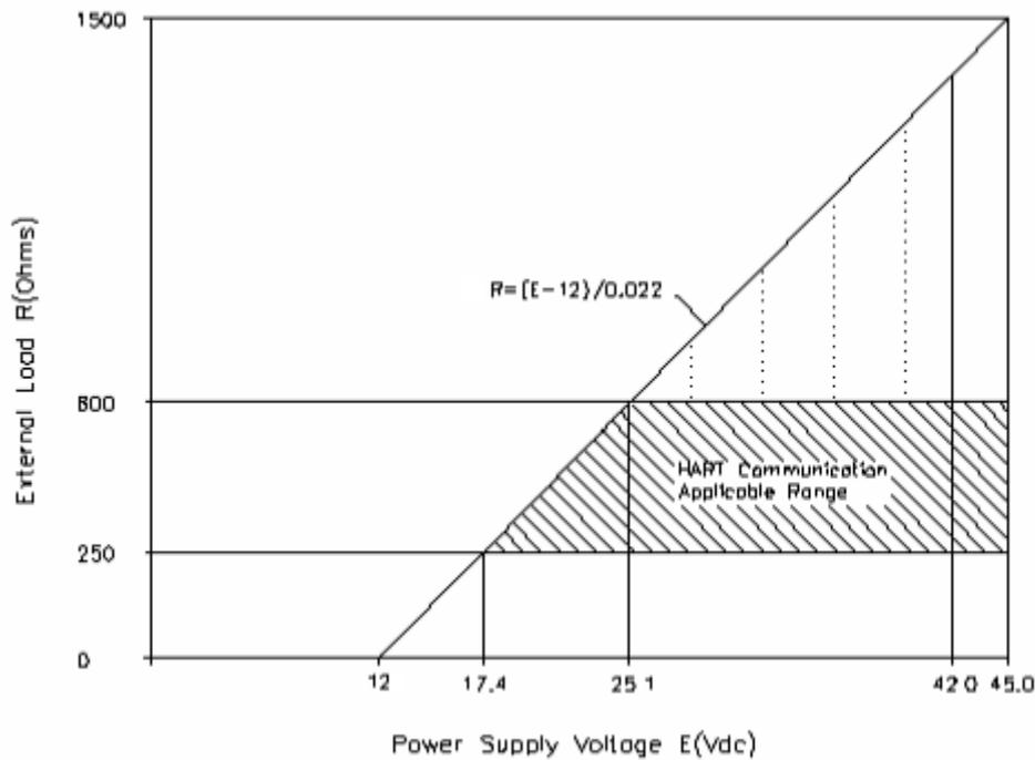
[Figure 5 Transmitter Power Limit Supply]
