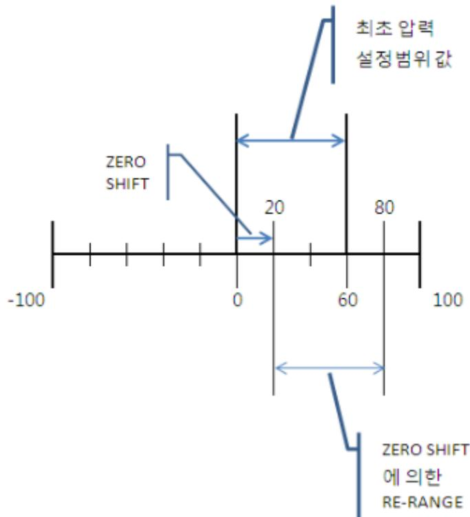
[Figure 6. Re-Range of ZERO SHIFT]
