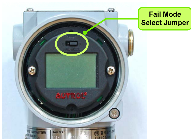
Figure 3-2 Fail Mode Selection Jumper Switch of LCD Module
